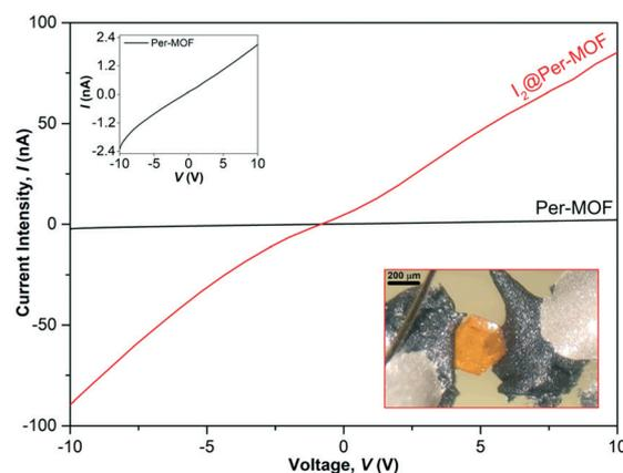
Fig. 7 Representative current ( $I$ )–voltage ( $V$ ) plot for crystal devices of **Per-MOF** (black) and  $I_2$ @**Per-MOF** (red) at 300 K. The inset in the upper panel shows the **Per-MOF**  $I$ – $V$  curve with a proper scale. The image in the lower panel shows a micrograph of an  $I_2$ @**Per-MOF** crystal with Ag epoxy + carbon-based paste contacts.
