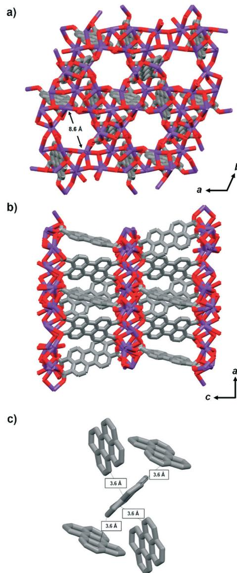
**Fig. 1** Crystal structure of **Per-MOF**: a) microporous channels along the *c*-axis, and b) packing of the perylene-based linkers along the *a*-axis. c) Partial view of the herringbone arrangement of the perylene-based linkers within the structure, showing the shortest C...C distances between neighbouring perylenes. Colour code: C (grey), O (red), K (purple). For simplicity, water molecules and hydrogens are omitted.
