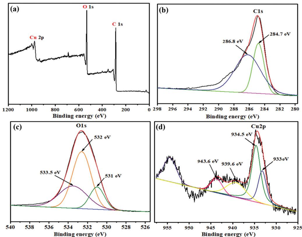
Fig. 6 XPS spectra of the CuO/rGO (CG-V) nanocomposite.
