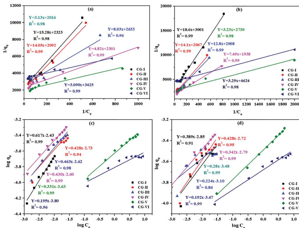
Fig. 8 (a and b) Langmuir adsorption isotherms and (c and d) Freundlich adsorption isotherms for  $\text{Bi}^{3+}$  and  $\text{Cd}^{2+}$  ion adsorption on different adsorbent samples of rGO, CuO and CuO/rGO nanocomposites.
