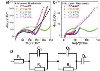
Fig. 10 Nyquist plots of Li-metal/LTO half-cells, before the rate test (a), and after the cycle test (b). The equivalent circuit (c) with  $R_1$  the apparatus resistance and two R-Q elements, the Li- metal/electrolyte and electrolyte/LTO interfaces.  $Q_4$  accounts for Li-ion diffusion at low frequencies.
