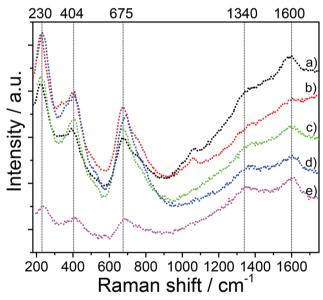
Fig. 3 Raman spectra of the mesoporous LTO microspheres. (a) LTO-A-600, (b) LTO-A-700, (c) LTO-B-600, (d) LTO-B-700, and (e) LTO-C-700.
