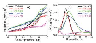
Fig. 5 (a) Nitrogen physisorption isotherms of the mesoporous LTO microspheres at 77 K. (b) Pore size distribution as determined from the adsorption branch using the BJH method, where the derivative pore volume normalised to the natural logarithm of pore-width interval, dV/  $d \log(W)$ , is shown as a function of the pore width.
