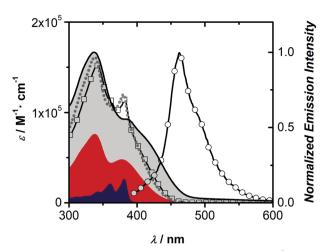
Fig. 3 Molar absorption coefficients in DCM of  $\mathbf{1}$  (squares,  $10^{-5}$  M) and its fluorescence spectrum (excitation 381 nm, circles) compared to building blocks PTZ 2 (red fill) and NDI 3 (blue fill) in DCM. The grey dashed line represents the addition of 2 and 3 in a 2:1 summative ratio and the black line (grey fill) represents the normalized solid-state film absorption profile of 1
