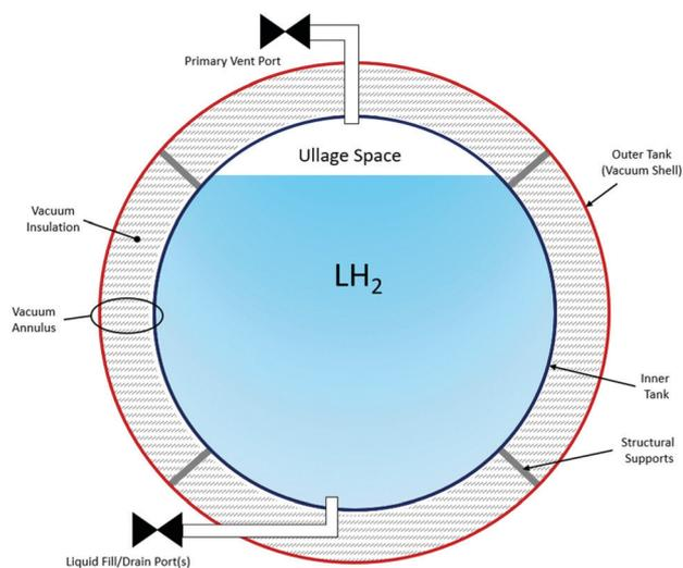
Fig. 15 A schematic showing general features of a LH<sub>2</sub> storage tank.
