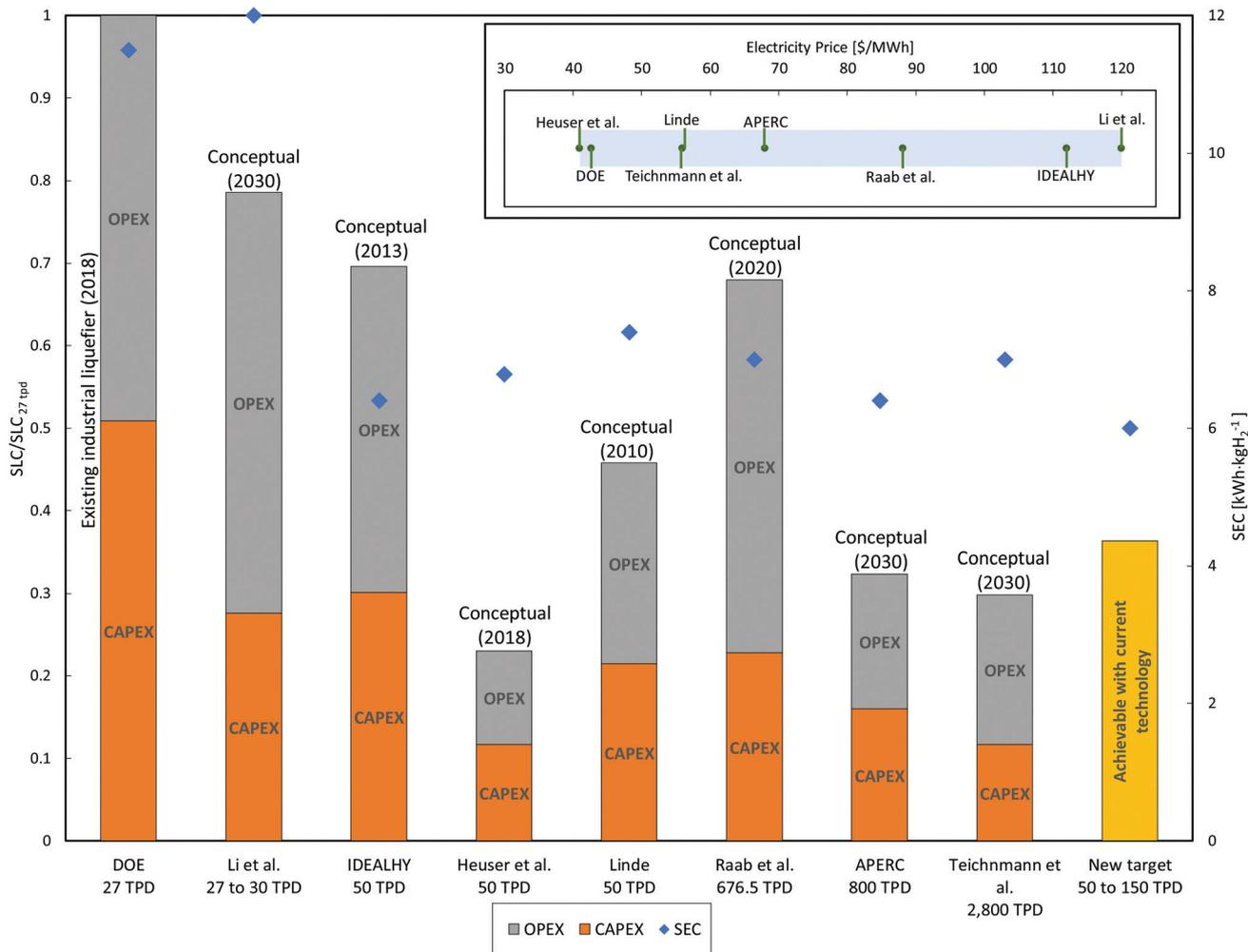
Fig. 14 Specific energy consumption (SEC) and specific liquefaction costs (SLC) relative to a reference 27 TPD  $\text{LH}_2$  process (\$2.75 per kg  $\text{H}_2$ ) and the various conceptual processes estimated at different electricity costs.
