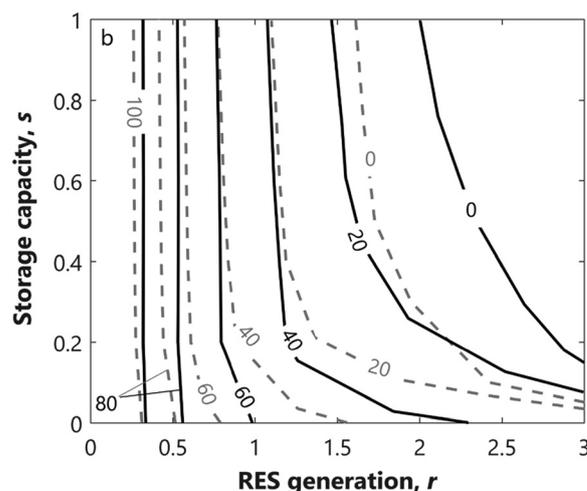
Fig. 1 CO<sub>2</sub> emissions isolines (in t per GWh<sub>e</sub>) at varying undispachable renewable generation (x-axis) and storage capacity (y-axis) when considering a system with only H<sub>2</sub> storage (solid lines) and H<sub>2</sub> storage + batteries (dashed lines). Adapted from Gabrielli *et al.*<sup>64</sup>
