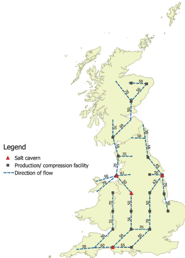
Fig. 12 Transmission of H<sub>2</sub> to supply peak heat demands for Great Britain based on Sunny *et al.*<sup>125</sup> The direction of transmission is illustrated with the numeric labels representing the average operating pressure of the transmission line measured in bar. Salt caverns and production facilities dispense H<sub>2</sub>, and booster compressors increase the transmission pressures to satisfy periods of high demand.
