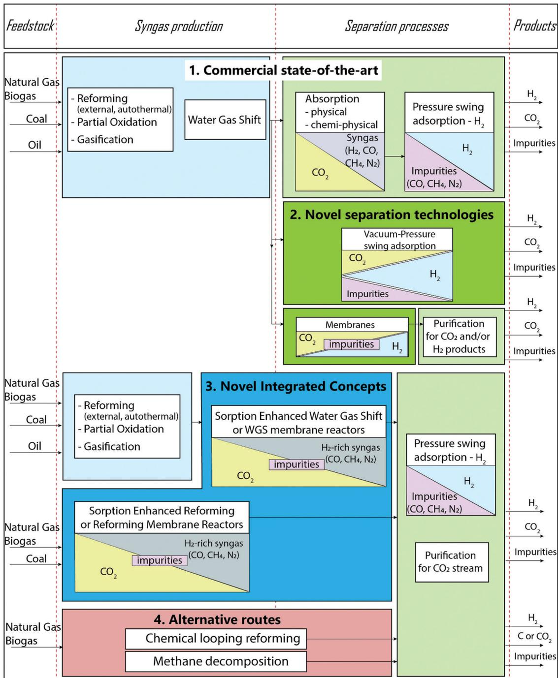
Fig. 9 Hydrogen production from fossil fuels with carbon capture and storage, with highlight on current and future pathways relevant for CO<sub>2</sub>-neutrality in 2050.
