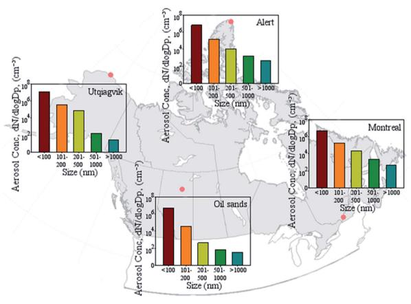
Fig. 4 Abundance of different size fractions in North American snow. Data obtained from references.  $^{1.102}$  The data was obtained using a scanning mobility particle sizer and an optical particle sizer with size limits from 11.5 to 9033.88 nm. Each color represents a different size fraction, which is on x-axis.
