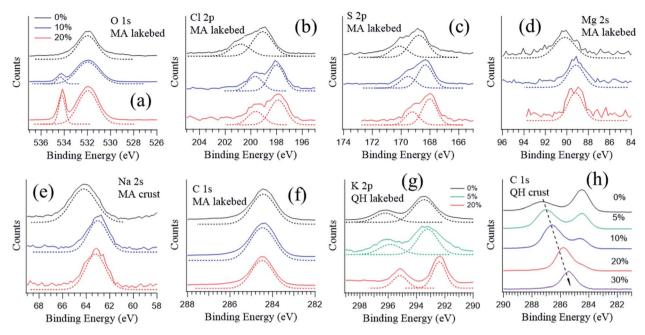
Fig. 4 Photoemission spectra of the MA lakebed samples at RH = 0% (black), 10% (blue), and 20% (red): (a) O 1s, (b) Cl 2p, (c) S 2p, (d) Mg 2s, (e) Na 2s and (f) C 1s. Photoemission spectra of (g) K 2p of the QH lakebed samples and (h) C 1s of the QH crust at different RHs. The photon energy was varied to yield an electron kinetic energy at 300 eV.
