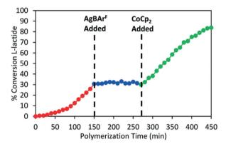
Fig. 3 Time vs. conversion plot of redox switchable ROP of L-LA using Zr complex 8b<sup>red/ox.50</sup> The oxidised species 8b<sup>ox</sup> was generated in situ by addition of AgBAr<sup>F</sup> (blue circles) and the reduced species was regenerated by CoCp2 (green circles). Reproduced from ref. 50 with permission from the Royal Society of Chemistry.
