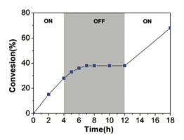
**Fig. 7** Time vs. conversion plot for ROP of VL in light on-off experiments.<sup>87</sup> Reproduced from ref. 87 with permission from the Royal Society of Chemistry.
