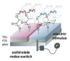
Fig. 5 Surface anchored bis(imino)pyridine iron catalysts for ROP allowing patterning of surfaces with polymer brushes through application of an electrical stimulus. 55 Reproduced from ref. 55 with permission from the Royal Society of Chemistry.
