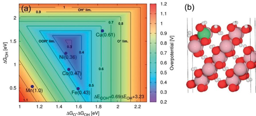
Fig. 42 (a) 2D map of theoretical overpotentials  $\eta$  for the doped  $10\bar{1}4$  surface of  $\beta$ -CoOOH as function of  $\Delta G_{\text{O}} - \Delta G_{\text{OH}}$  and  $\Delta G_{\text{OH}}$ . The individual values of  $\eta$  are indicated in brackets. Improvement in activity relative to undoped surface is obtained in the case of Ni with  $\eta = 0.36$  V and Fe with 0.43 V. Reproduced with permission from ref. 711. Copyright American Chemical Society 2013.
