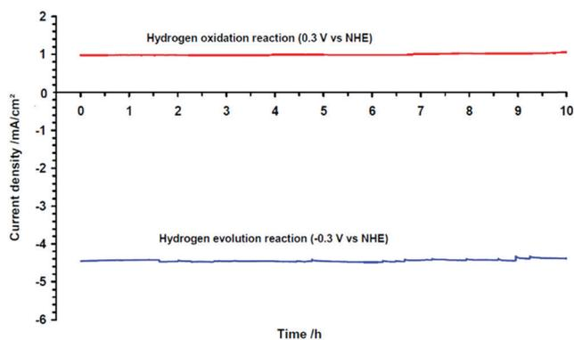
Fig. 137 Long-run electrolysis experiments for both hydrogen evolution and oxidation carried out respectively at  $-0.3$  and  $+0.3$  V vs. NHE in H<sub>2</sub>SO<sub>4</sub> (0.5 mol L<sup>-1</sup>) on a membrane electrode on which MWCNTs have been deposited and further Ni-functionalised. Reprinted with permission from ref. 1677 Copyright 2009 AAAS.
