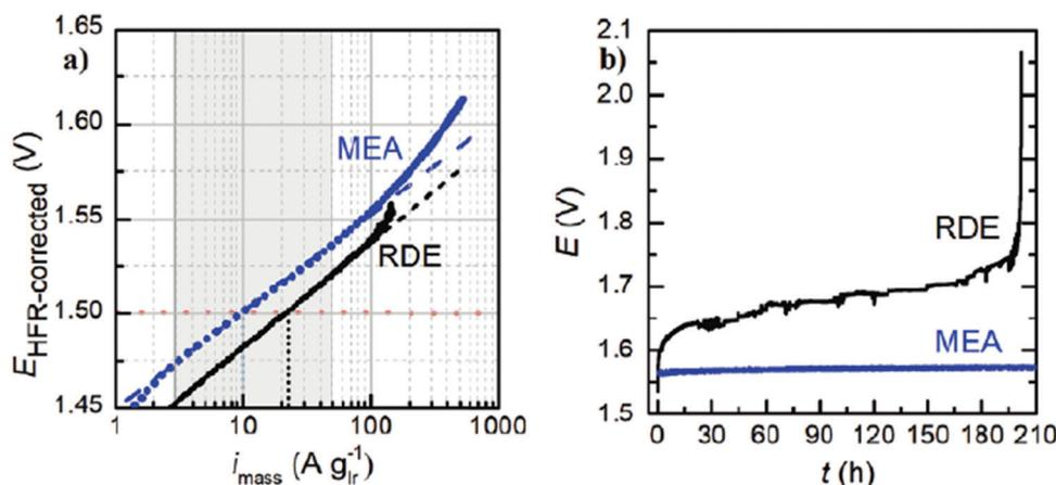
Fig. 144 Evaluation of the OER (a) activity and (b) stability versus time at a given representative OER current in MEA (blue) and RDE (black) configuration for a state-of-the-art commercial  $\text{IrO}_2$  catalyst. Reproduced from ref. 20 with permission from Wiley.
