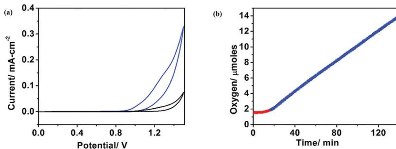
**Fig. 128** Cyclic voltammograms (V vs. Ag/AgCl) of Nafion films, loaded (blue trace) and not loaded (black trace) with  $\text{Fe}(\text{tpfc})\text{Cl}$ , on FTO electrodes in pH 10 phosphate–KOH buffer (scan rate of  $100 \text{ mV s}^{-1}$ ; catalyst loading  $1.6 \text{ nmol cm}^{-2}$ ). (b) Evolution of oxygen before (red) and after (blue) application of a potential of 1.5 V. Reprinted with permission from ref. 1577 Copyright 2020. American Chemical Society.
