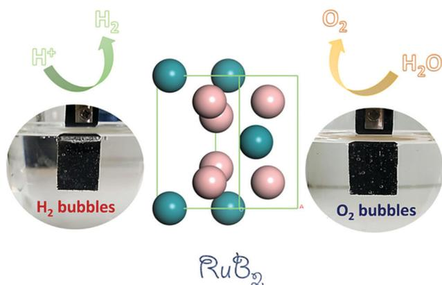
**Fig. 57** Schematic representation of the use of RuB<sub>2</sub> as an anode and cathode in a water electrolysis approach. Reproduced with permission from ref. 949. Copyright American Chemical Society 2020.
