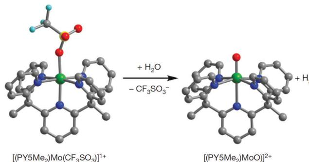
Fig. 138 Reaction of [(PY5Me<sub>2</sub>)Mo(CF<sub>3</sub>SO<sub>3</sub>)]<sup>+</sup> with water to form [(PY5Me<sub>2</sub>)MoO]<sup>2+</sup> and release H<sub>2</sub>. Reprinted with permission from ref. 1679. Copyright 2010. Nature publishing.
