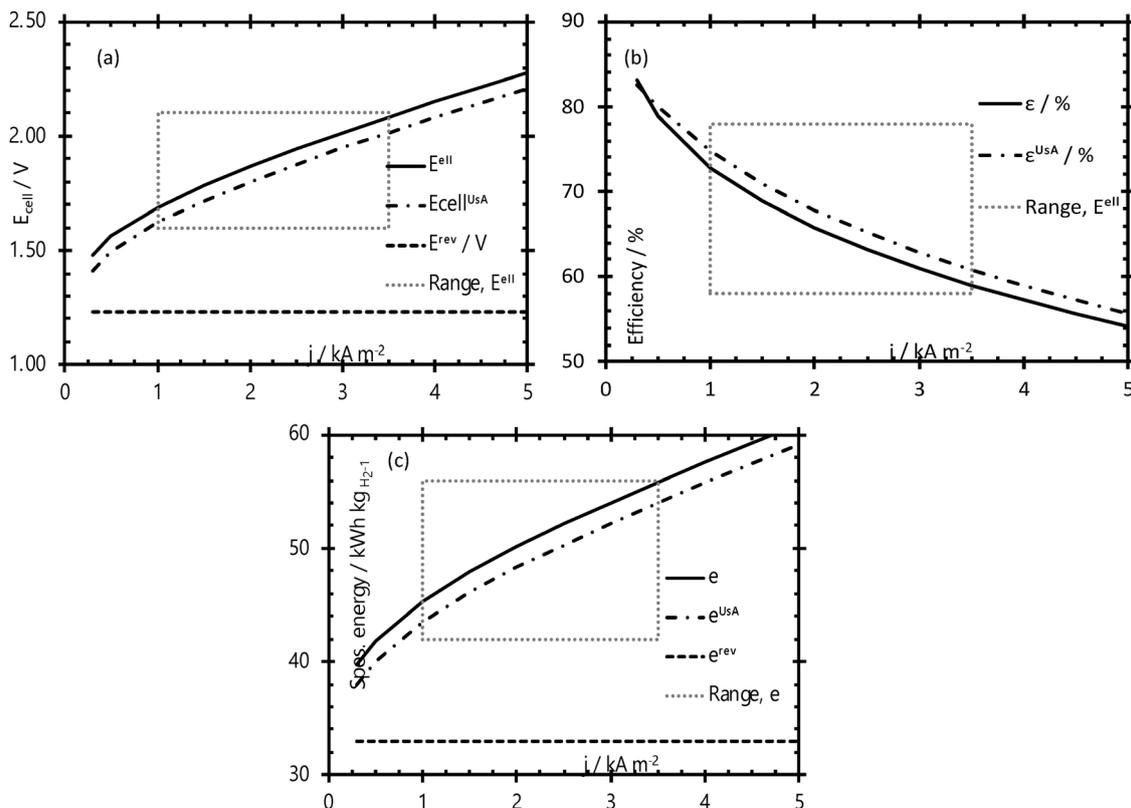
Fig. 148 Effect of ultrasound on (a) cell voltage ( $E_{\text{cell}}$ ), (b) efficiency ( $\epsilon$ ) and (c) specific energy ( $e$ ) for hydrogen production (\*UsA = ultrasound-assisted).<sup>1841</sup>
