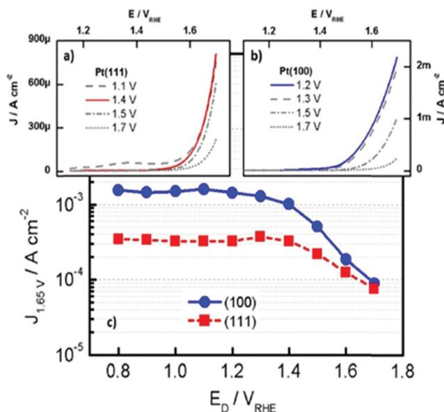
**Fig. 19** LSV curves of (a) Pt(111), (b) Pt(100) in 0.1 M HClO<sub>4</sub> with scan rate of 50 mV s<sup>-1</sup>. (c) Plot of the current density at +1.65 V vs. RHE (*j*<sub>+1.65V</sub>) in the LSV as a function of the applied potential. Reproduced with permission from ref. 427. Copyright Wiley 2019.
