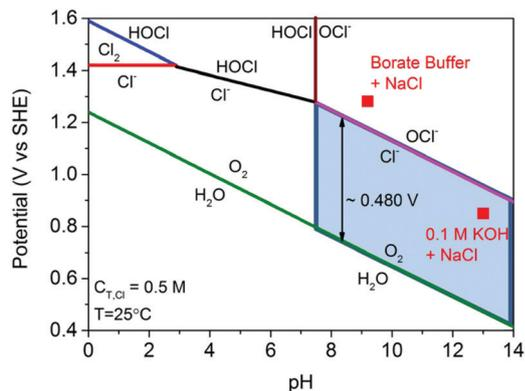
**Fig. 150** Pourbaix diagram for electrolysis of 0.5 M NaCl. The electrode potential for OER is included as well, assuming oxygen partial pressure of 0.021 MPa. The red square points show the operating potentials (vs. SHE) after 1 h constant current density of 10 mA cm<sup>-2</sup> with NiFe LDH catalyst in 0.1 M KOH + 0.5 M NaCl (pH 13) and 0.3 M borate buffer + 0.5 M NaCl (pH 9.2) electrolyte. Reproduced with permission from ref. 1864 Copyright Wiley 2016.
