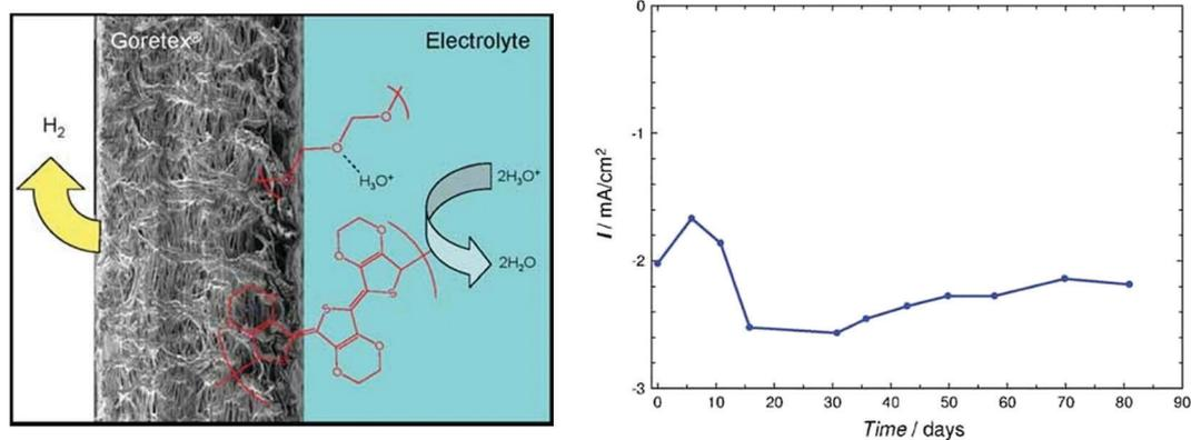
Fig. 94 Schematic of PEDOT-based HER electrode (left side). Long-term performance of PEDOT-PEG on Goretex/Au in 1 M  $\text{H}_2\text{SO}_4$  under  $\text{N}_2$  at  $-0.35$  V vs. SCE. Reproduced with permission from ref. 1339. Copyright 2010 Wiley.
