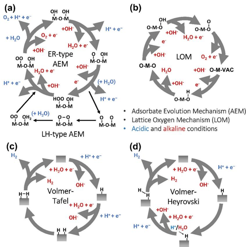
**Scheme 1** (a) The acid–base and direct coupling adsorbate evolution reaction mechanisms of OER in the acidic (blue) or alkaline (red) medium. (b) The lattice oxygen mechanism of OER in alkaline medium. (c) The Volmer–Tafel HER mechanism on the electrode surface in acidic (blue) or alkaline (red) conditions. (d) Volmer–Heyrovsky mechanism of the HER.
