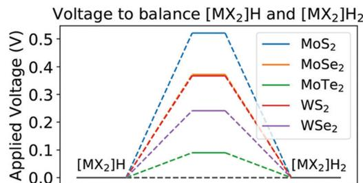
Fig. 77 Required applied potential to obtain a zero-reaction energy for the rate determining Volmer step from [MX<sub>2</sub>]H to [MX<sub>2</sub>]H<sub>2</sub>. Reproduced with permission from ref. 1138 Copyright 2018 American Chemical Society.
