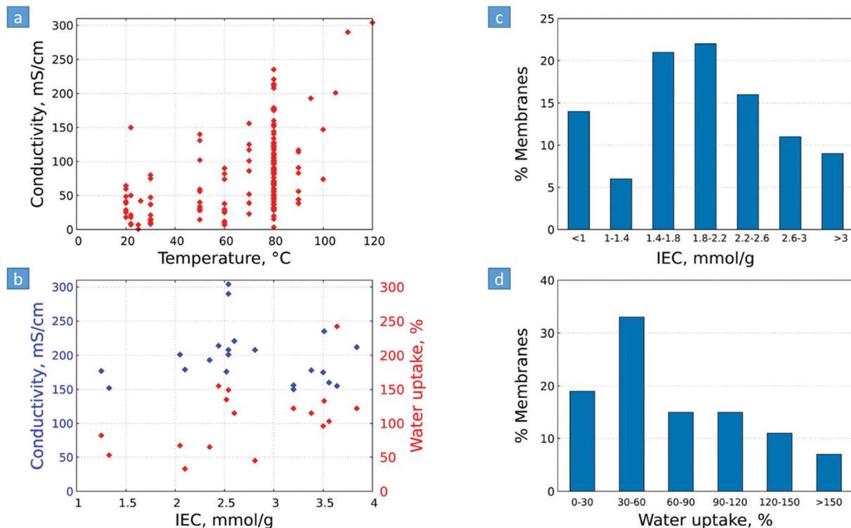
Fig. 10 (a) AEM hydroxide conductivity vs. temperature, and (b) hydroxide conductivity and water uptake of selected AEMs (with conductivities  $\geq 150 \text{ mS cm}^{-1}$ ). (c) Fraction of AEMs at different levels of (c) IEC range and (d) water uptake range. Water uptake values are given in different temperatures. Represented data and the underlying sources are given in Table S1 (ESI<sup>†</sup>).
