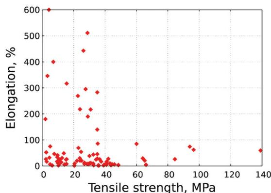
Fig. 14 Elongation [%] vs. tensile strength [MPa]. In case there is a range of values, the lower value was considered. Represented data and underlying sources are given in Table S1 (ESI<sup>†</sup>).
