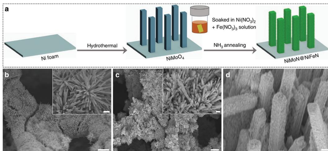
Fig. 70 Synthesis and microscopic characterisation of the as-prepared NiMoN@NiFeN catalyst. (a) Schematic illustration of the synthesis procedures for the self-supported 3D core-shell NiMoN@NiFeN catalyst. (b–d) SEM images of (b) NiMoN and (c and d) NiMoN@NiFeN at different magnifications. Reproduced with permission from ref. 1044 Copyright Nature Publishing 2019.
