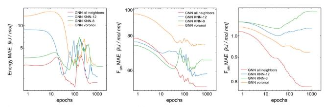
Fig. 7 Learning curves on the validation set of the  $\Delta$ -learning GCNN model when using different neighborhood selection schemes. The test system uracil in water was used.
