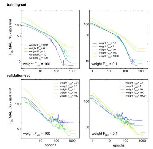
Fig. 6 Learning curves of  $F_{\text{OM}}$  in the training set (top) and validation set (bottom) when varying the relative loss weightings  $wF_{\text{OM}}$  (left) and  $wF_{\text{MM}}$  (right). The basic GCNN with the Δ-learning scheme and the test system uracil in water was used. The weight of the energy loss (wE) is kept constant at 1.0.
