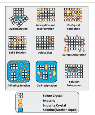
Fig. 1 Schematic illustration of the different impurity incorporation mechanisms in solution crystallization. Inspired by Urwin et al. and expanded for this work.44
