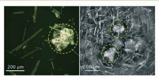
Fig. 3 Optical microscopy (left) and in situ process images (right) of co-precipitates of phenylglycine impurities (circled) crystallization of needle-like cephalexin monohydrate crystals [adapted with permission from Salami et al.77 Copyright 2021 American Chemical Society].
