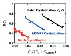
**Fig. 8** Fits to eqn (2) for the experimental distribution coefficients of an enone impurity for the nominal concentration level in batch crystallization (red), the nominal concentration level in continuous crystallization (blue), and three times the nominal concentration level in batch crystallization (black) [adapted with permission from Maloney et al.<sup>25</sup> Copyright 2020 American Chemical Society].
