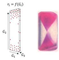
Fig. 2 Left: Face-dependent crystal growth (Gi) and impurity incorporation (ri) in a growing crystal. Right: Example of facedependent incorporation of sulforhodamine B in a K<sub>2</sub>SO<sub>4</sub> crystal [adapted with permission from Kahr and Gurney.<sup>54</sup> Copyright 2001 American Chemical Society].
