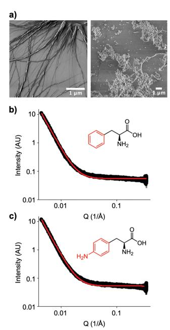
Fig. 4 Amino acid self-assembly. (a) SEM images of L-phenylalanine (left) and 4-amino-L-phenylalanine (right) from 6 mM solutions; (b) SAXS spectra of Phe; (c) SAXS spectrum of amino-phe. SAXS conducted at 1.5 mg mL $^{-1}$ . Black line is data and red line is fit to a power law model.
