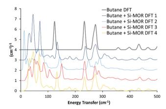
Fig. 2 Comparing the calculated INS spectra of n-butane in siliceous mordenite for a range of geometries. In all cases, the experimental shifts of the butane torsional modes to lower energy values, on encapsulation in the mordenite pore (Fig. 1) were not replicated. See text for further details. Data is artificially incremented by  $1 (cm^{-1})^{-1}$  for ease of reading.
