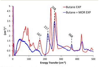
Fig. 1 The difference in the experimental INS spectra on encapsulating butane into commercial mordenite (Butane + MOR EXP), compared to pure *n*-butane (Butane EXP), for <500 cm<sup>-1</sup>
