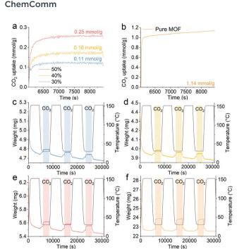
Fig. 3 CO<sub>2</sub> capture performance of (a) hybrid aerogels with different MOF loadings and (b) pure MOF, (c-f) weight changes for three consecutive cycles of CO<sub>2</sub> sorption-desorption of hybrid aerogels with 30%, 40%, 50% MOF and pure MOF, respectively.
