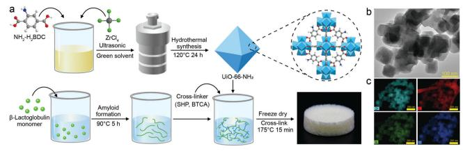
Fig. 1 Fabrication process of hybrid UiO-66-NH2 and amyloid fibrils aerogel. (a) Schematic of UiO-66-NH2 synthesis, and the preparation process of the hybrid aerogel. Morphological features of UiO-66-NH<sub>2</sub>. (b) TEM image of UiO-66-NH<sub>2</sub>. (c) Elemental maps of UiO-66-NH<sub>2</sub>.
