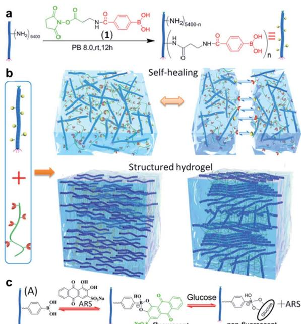
Fig. 17 (a) Preparation of PBA–M13. (b) Hydrogel prepared using PBA–M13 and PVA, and its self-healing behavior. (c) Fluorescence-on behavior upon the binding of ARS to PBA–M13 and its fluorescence-off behavior upon exchange with glucose. Reproduced from ref. 95 with permission from the ACS.
