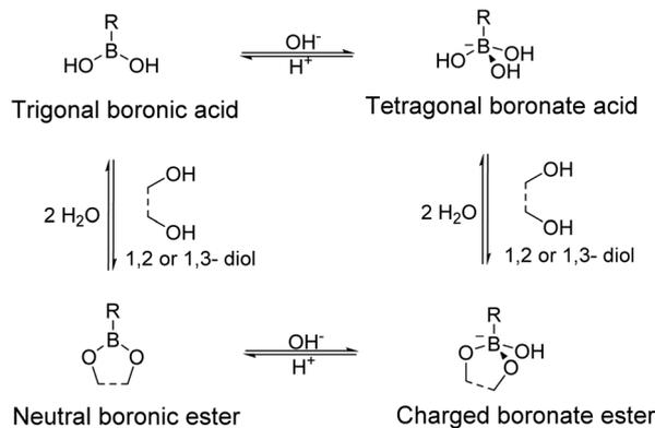
Fig. 2 Dynamic equilibrium of boronic acid with 1,2- or 1,3-diols in an aqueous solution.
