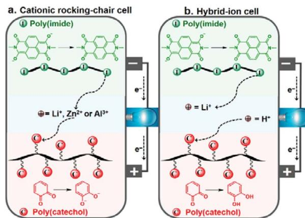
Scheme 1 Schematic of the working principle of the PI-PC full-cell during the discharge process in a cationic rocking-chair mode with Li<sup>+</sup>, Zn<sup>2+</sup> or Al<sup>3+</sup> (a), and hybrid-ion configuration with Li<sup>+</sup>/H<sup>+</sup> (b).
