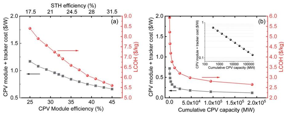
Fig. 4 (a) Module + tracker costs (left) and cost of H<sub>2</sub> (right) as a function of CPV module efficiency (bottom) and STH efficiency (top). (b) Module + tracker costs (left) and cost of H<sub>2</sub> (right) as a function of projected cumulative CPV capacity (bottom). For both projections, the electrolyser efficiency, CAPEX and OPEX were kept constant as mentioned in Tables 2 and 3.
