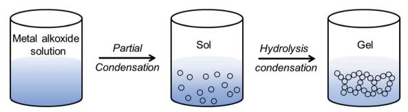
Fig. 4 Schematic of sol-gel synthesis used for the ceramic materials. Metal alkoxide (M-O-R; where R is alkyl or aryl group) is formed *via* dissolution of metal salts in alcohol. Hydrolysis and partial condensation of metal alkoxide leads to 'sol' formation, which upon further heating undergoes polycondensation to form a three-dimensional gel network. The gel can be transformed into powdered product upon high temperature decomposition and calcination.
