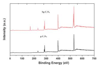
Fig. 8 XPS survey scans of g-C<sub>3</sub>N<sub>4</sub> and Sg-C<sub>3</sub>N<sub>4</sub>.
