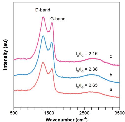
Fig. 5 Raman spectra of (a) 0.01Li-F-PCNFs, (b) 0.05Li-F-PCNFs, and (c) 0.1Li-F-PCNFs composites.
