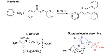
Scheme 20 The IL-catalysed aza-Michael reaction and supramolecular assembly formed following the interaction between the IL and starting materials. Supramolecular interactions are represented by dashed lines.
