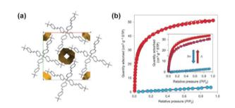
Fig. 12 (a) Packing of the tetrameric azobenzenes in the solid state along with representation of the empty channels. (b)  $CO_2$  adsorption isotherms at 195 K of pristine material (red isotherm) and after exposure to UV light (blue isotherm). Reprinted by permission from Springer Nature from ref. 115, Copyright 2015.
