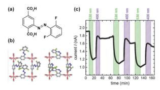
Fig. 23 (a) Structure of ortho-fluoro azobenzene linkers and (b) switchable SURMOF viewed in c direction. (c) Changes in the proton current conduction of butanediol in SURMOF at 1 V and 1 Hz upon alternating irradiation at 530 and 400 nm. Adapted with permission from ref. 145. Copyright 2018 Wiley-VHC.
