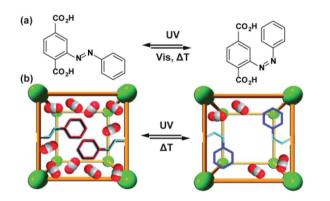
Fig. 7 (a) Structure and switching of the incorporated azobenzene in the isoreticular MOF-5 scaffold. (b) Schematic depiction of the light and heat induced structural changes in the pore structure and gas adsorption of azobenzene functionalized isoreticular MOF-5 structural reprinted with permission from ref. 105 Copyright 2013 American Chemical Society.
