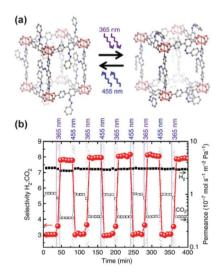
Fig. 11 (a) Representation of light induced structural changes in the SURMOF functionalized with azobenzene pendants. (b) Light-induced changes in selectivity of  $\rm H_2/CO_2$  separation on  $\alpha\text{-Al}_2\rm O_3\text{-supported}$  SURMOF membrane (red circles) and  $\rm H_2$  (black squares) and  $\rm CO_2$  (white squares). Adapted by permission from Springer Nature from ref. 126, Copyright 2014.
