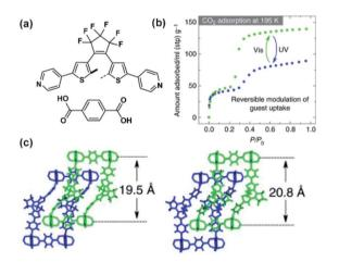
Fig. 15 (a) Structure of the linkers used to construct two-fold interpenetrated framework. (b) CO<sub>2</sub> adsorption isotherms of pristine (green points) and irradiated (blue points) materials. (c) Representation of the SC X-ray structure of pristine (left) material and UV-treated (right) materials viewed along b direction. Adapted by permission from Springer Nature from ref. 121, Copyright 2017.
