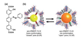
Fig. 18 (a) Structural the azobenzene linker. (b) Schematic representation of light-induced changes in pore aperture of MOF-74 upon photochemical isomerization of the appended azobenzenes. Adapted with permission from ref. 128. Copyright 2013, Royal Society of Chemistry.
