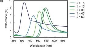
Fig. 5 (a) Photographs at different viewing angles of films prepared from aqueous dispersions of Wp2 with various amounts of Bp1-h. (b) Absolute specular reflectance UV-vis spectra of a cast film containing Wp2 and 5 wt% of Bp1-h. Both the incident angle and the detection angle were set to the specified angles ( $\theta$ ).
