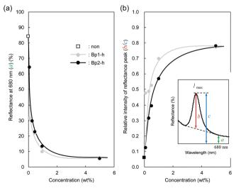
Fig. 4 (a) Baseline reflectance (680 nm, a) and (b) the relative peak intensity at  $\lambda_{\rm max}$  (b/c) after doping black carbon nanoparticles at different concentrations.
