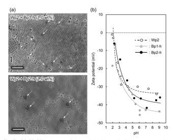
Fig. 3 (a) FE-SEM images of the colloidal crystal of silica nanoparticles (Wp2) with 1 wt% black carbon nanoparticles (Bp1-h and Bp2-h). Scale bars: 2 µm. (b) Zeta potentials of the aqueous dispersions of Wp1, Bp1-h, and Bp2-h in a wide pH range
