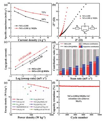
(a) Specific capacities at different current densities and (b) Nyquist plots of Ni-Co LDH and Ni-Co LDH@MQDs. (c) Plots of log(i) versus log(v) of the samples. (d) The capacitive- and diffusion-controlled processes for Ni-Co LDH@MQDs at different scan rates. (e) Ragone plots. (f) Cycling performance of Ni-Co LDH@MQDs//AC at a current density of 6 A g<sup>-1</sup>.
