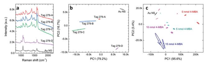
Fig. 4 (a) SERS spectra of AuNS and tag 279 with different concentrations of MG. (b) The PCA score plot of the SERS spectra, where each sample was measured five times. (c) The PCA score plot of a series of tags with different concentrations of 4-MBA and MG. In each color set, the amounts of MG are 0, 1, 2, and 3 nmol in 1 mL of solution (lighter to darker color).
