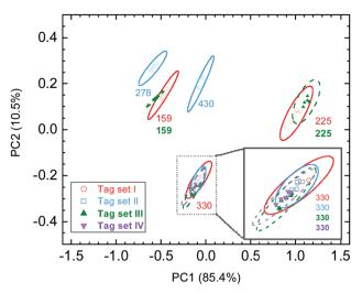
Fig. 3 PCA score plot of four tag sets with various tag IDs. All the tag sets included a common tag 330. Tag sets I and II (open circles and squares) were associated with one batch of AuNSs while tag sets III and IV (closed triangles) were associated with different batches of AuNSs. A zoom-in for tag 330 was given in the inset for a clearer view.
