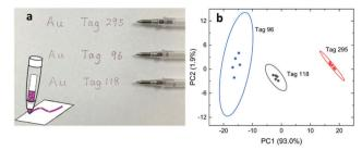
Fig. 6 (a) An image of a paper written using three different SERS inks and the ballpoint pens containing the inks. Inset: A schematic of SERS ink contains AuNSs and chemicals that could be written on paper. (b) The PCA score plot of the Raman spectra of the written patterns, where a 1064 nm laser, a 1 second exposure time, and a laser intensity of 20% were used.
