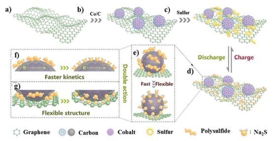
Fig. 8 Schematic illustration of the S@Co/C/rGO electrode design. (a-c) Illustration of the synthesis. (d-g) Advantages of the S@Co/C/rGO composite. Reproduced with permission. 110 Copyright 2020, Elsevier.
