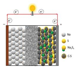
Fig. 2 Schematic representation of an RT-Na/S battery.
