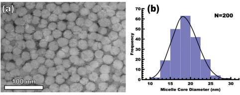
Fig. 4 TEM image of OS1-EtOH micelles (a) and the associated micelle core size distribution (b). The mean diameter and standard-error-of-the-mean of the measured cores are 18.68 and 0.22 nm, respectively (Table S1, ESI†). The PEO corona was selectively stained with 1 wt% uranyl acetate for contrast (dark) relative to the unstained PS (light)
