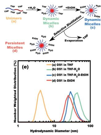
**Fig. 3** Schematic representation of glassy-PMT preparation with the polymer OS1. DLS after polymer dissolution in a good solvent, THF (a), reveals unimers in solution. Poor-solvents are next added where first water induces micellization (b) before a large excess of ethanol is added (c). The THF is then removed by rotary evaporation to yield micelles that are dispersed in purely poor-solvents for the core block (d). DLS data (e) show the hydrodynamic diameter at each stage of processing.
