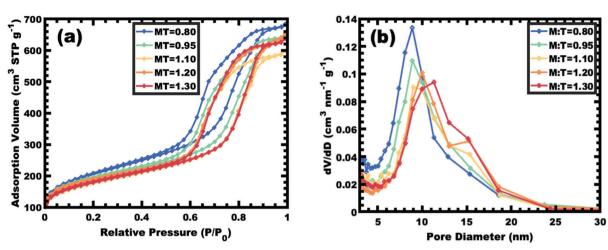
Fig. 10 Nitrogen physisorption isotherms for select samples from series OS1–EtOH (a) along with the corresponding BJH pore size analysis from the adsorption branch of the isotherm (b).
