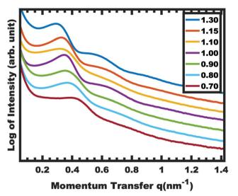
Fig. 8 SAXS of carbonized OS1-EtOH samples with increasing material: template ratio. The shift in peak position to lower q-values corresponds to an increase in d-spacing  $(2\pi/q)$ . The data were offset vertically for clarity.
