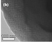
Fig. 1 SAXS (a) and TEM (b) data from representative sample OS1-EtOH-1.00 after carbonization. The inset 2D SAXS pattern has a color scale corresponding to the log of X-ray intensity. The momentum transfer  $q = 4\pi \sin(\theta)/\lambda$ , where  $2\theta$  is the total scattering angle and  $\lambda$  is the wavelength. The bright field TEM image shows the location of carbon (dark) and porosity (light).
