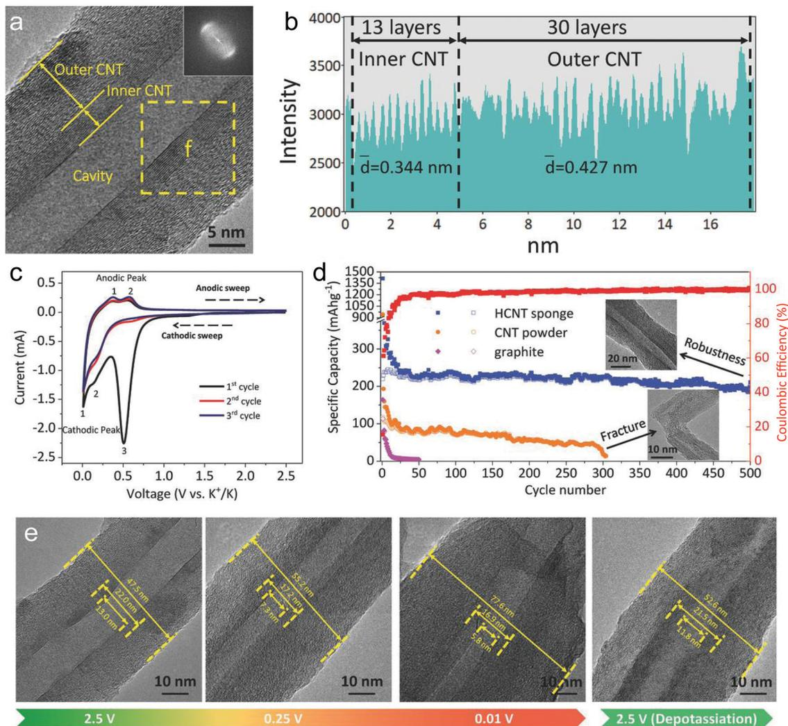
Fig. 20 (a) TEM image of a CNT. (b) Line profile obtained from the wall of a CNT. (c) CV curves of CNT sponge at  $0.3 \text{ mV s}^{-1}$ . (d) Cycling performance of CNT sponge, commercial CNT powder and graphite electrodes at a current density of  $100 \text{ mA g}^{-1}$ . (e) *Ex situ* TEM images of the CNT structure at different potassiation and de-potassiation potential in the first cycle. Reproduced from ref. 344 with permission from Wiley-VCH.
