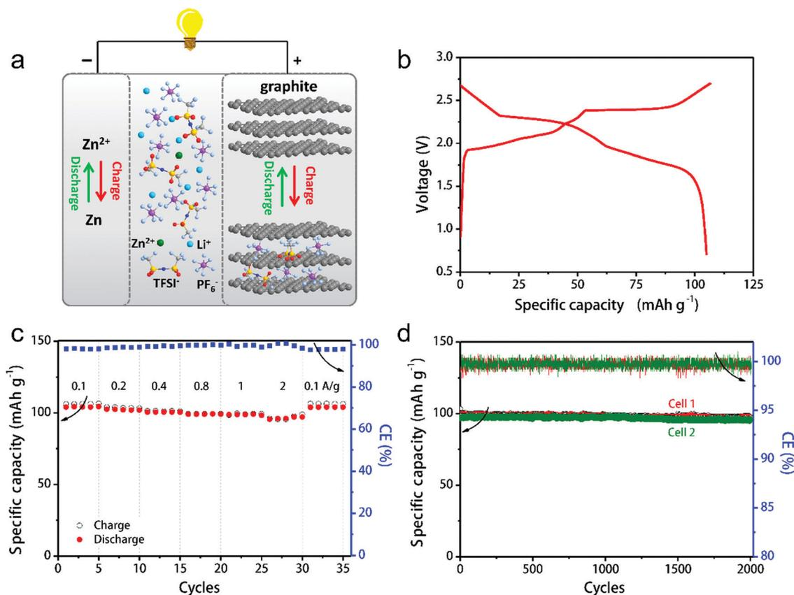
Fig. 31 (a) Schematic illustration of the Zn-graphite battery configuration and electrode reactions. (b) Typical charge-discharge curve at  $100 \text{ mA g}^{-1}$ , (c) rate capability and (d) cycling performance of the Zn-graphite battery at  $1000 \text{ mA g}^{-1}$ . Reproduced from ref. 431 with permission from Wiley-VCH.
