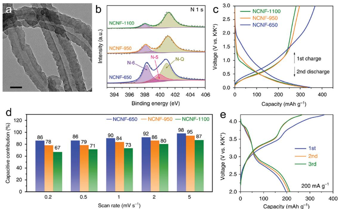
Fig. 24 (a) TEM of NCNF-650. (b) N 1s core level XPS high-resolution spectra, (c) first charge and second discharge profiles, and (d) contribution of the surface process at different scan rates of NCNF-650, NCNF-950, and NCNF-1100. (e) Galvanostatic charge/discharge profiles of the NCNF-650//Prussian blue full cell. Reproduced from ref. 360 with permission from Springer Nature.
