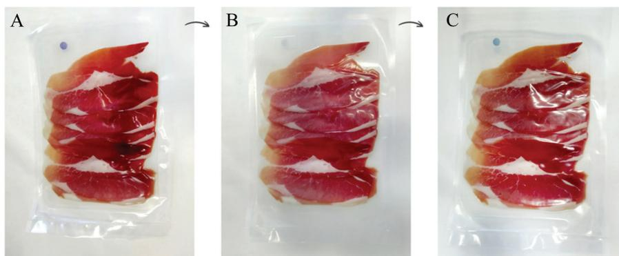
**Fig. 5** Photographs of UVA-activated oxygen indicator placed inside a plastic package flushed with CO<sub>2</sub> and sealed: (A) the package is recently sealed and the indicator is blue; (B) the indicator has been bleached by a UVC light burst, the indicator inside remains bleached for 48 h; and (C) upon opening the package, the entrance of oxygen causes the indicator to recover its original colour.
