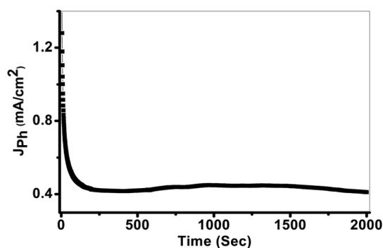
Fig. 8 Current–time characteristic under white light illumination.
