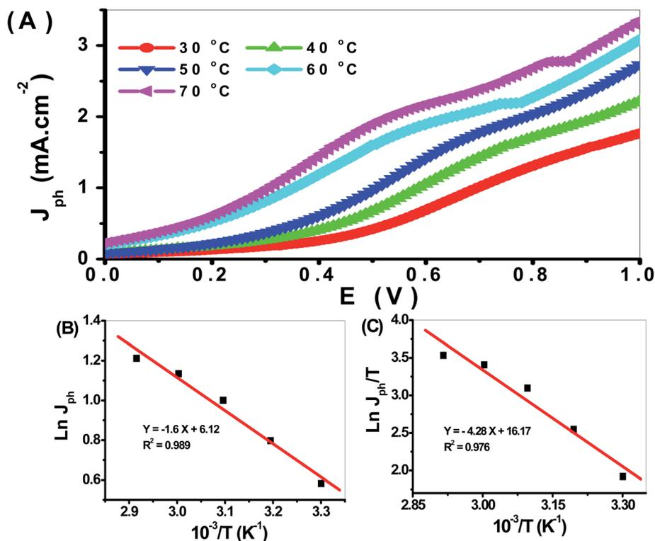
Fig. 11 (A) The effect of temperature on H<sub>2</sub> generation process, (B) plot of the  $J_{ph}$  against reciprocal of temperature, and (C) plot of  $J_{ph}/T$  versus reciprocal of reciprocal temperature.
