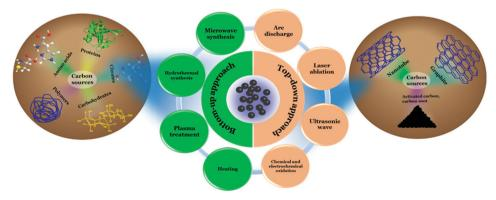
Fig. 1 Schematic illustration corresponding to different synthetic approaches used for Cdot preparation.
