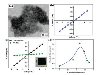
Fig. 7 (a) TEM image of the Cdot-PPy nanocomposite material. Plots of I-V characteristics corresponding to (b) Cdot film and (b) Cdot-PPy and PPy films. (d) Change in the conductivity of the composite due to the variation of Cdot content in the composite film. Reprinted with permission from ref. 119. Copyright 2016 American Chemical Society.
