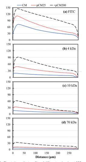
Fig. 8 The static gradient profiles of different molecules at 600 seconds in the middle channels of devices with parallel CM, pCM25 or pCM200: (a) FITC, (b) 4 kDa dextran, (c) 10 kDa dextran, and (d) 70 kDa dextran.
