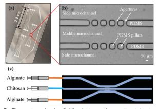
Fig. 3 Three-channel microfluidic device and experimental setup to generate static gradients. (a) A device with three sets of PDMS microchannels bonded to a  $3'' \times 1''$  glass slide; (b) zoom-in view of the aperture area of one microchannel network; and (c) experimental process to pump alginate and chitosan or chitosan with the nanoparticle solution into the microchannels for the biofabrication of parallel and semipermeable biopolymer membranes.
