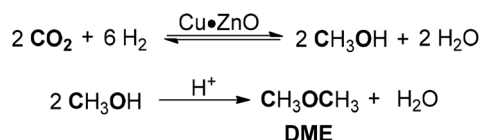
Scheme 20 Cu–ZnO-catalyzed synthesis of DME from CO 2 hydrogenation.
