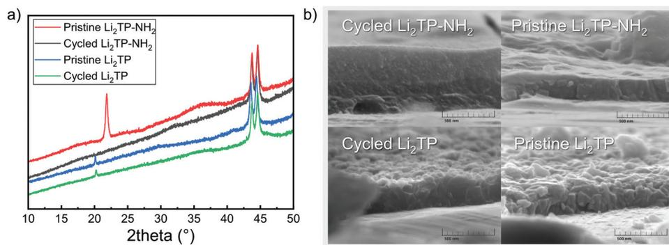
**Fig. 9** (a) Diffraction patterns of Li<sub>2</sub>TP-NH<sub>2</sub> (the shift in baseline and peaks at 44° are due to steel substrate), and (b) SEM images for a pristine and cycled Li<sub>2</sub>TP-NH<sub>2</sub> and Li<sub>2</sub>TP electrodes.
