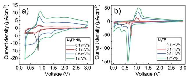
Fig. 6 Cyclic voltammograms for (a)  $\text{Li}_2\text{TP-NH}_2$  (0.25–3.0 V), and (b)  $\text{Li}_2\text{TP}$  (0.01–3.0 V) with various scan rates. The dark grey line represents the 1<sup>st</sup> cycle, and the red, blue, and green lines represent the subsequent cycles. Each cycle starts at the original open circuit voltage, being ca. 2 V for both the samples.
