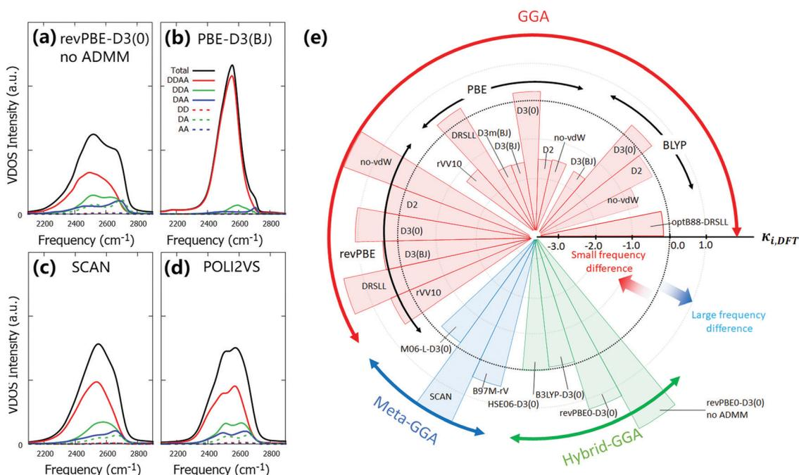
**Fig. 3** Decomposed VDOS spectra (a) at the revPBE0-D3(0) without ADMM level of theory, (b) at the PBE-D3(BJ) level of theory, and (c) at the SCAN level of theory as well as (d) with the POLI2VS model. (e) Pie chart of averaged  $\kappa_{i,DFT}$  for various DFT methods.
