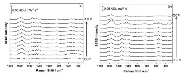
Fig. 4 (a) EC-SERS signal for THC-COOH on the AqNP-modified SPE at OCP, and then from 0.0 to -1.0 V in 100 mV increments. (b) EC-SERS signal stepping back from -1.0 V to 0.0 V in 100 mV increments, and finally at OCP measured after the potential stepping. Spectra measured at 780 nm, 80 mW, 30 seconds.
