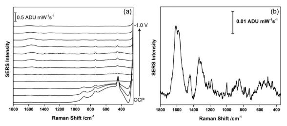
Fig. 6 (a) EC-SERS progression (cathodic) starting at OCP, and then stepping from 0.0 V to -1.0 V in 100 mV increments for THC drop-coated onto the electrode surface and then measured in artificial saliva. (b) EC-SERS signal recorded at -1.0 V vs. Ag/AgCl. Spectra measured at 780 nm, 80 mW, 30 seconds.
