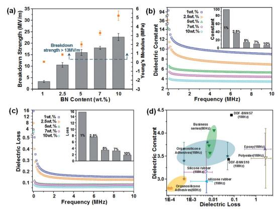
Fig. 4 (a) The breakdown strength of DDF-BNNS with different BNNS-NH<sub>2</sub> content. The frequency-dependent dielectric constant (b) and loss (c) of DDF-BNNS with different BNNS-NH2 content; inset: dielectric constant (b) and loss (c) of DDF-BNNS with different BNNS-NH2 content at 20 MHz. (d) A comparison of dielectric constant and loss values between different adhesives and insulating materials.
