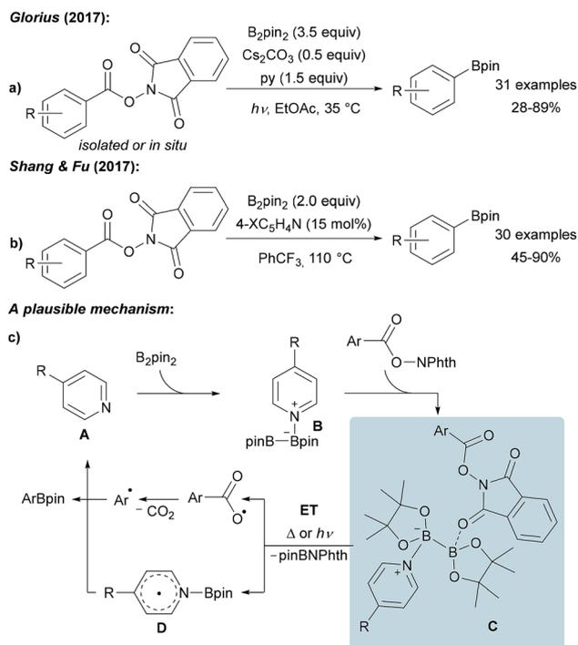
Scheme 12 Decarboxylative borylation of NHPI esters using  $B_2pin_2$  under basic conditions and irradiation with blue LEDs (a) or mediated by *tert*-butyl nicotinate ( $X = tBuO_2C$ , (b)). Mechanism (c).
