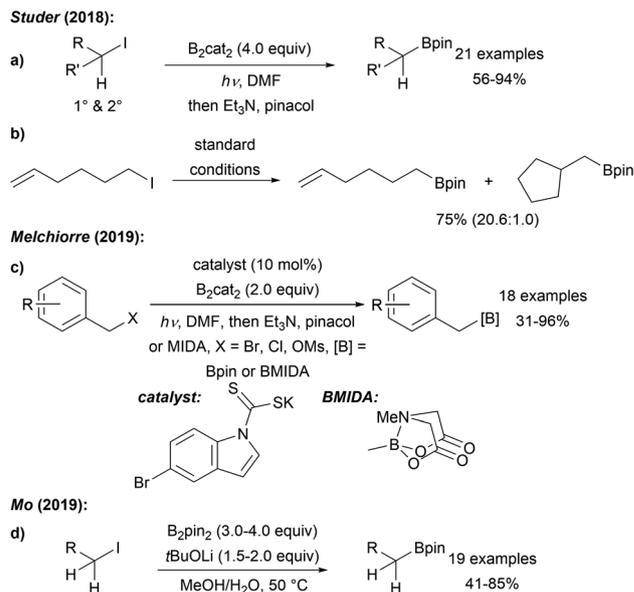
**Scheme 16** Metal free radical borylation of alkyl iodides (a) and radical probe experiment (b). Dithiocarbonyl anion enabled borylation of benzyl electrophiles (c) using  $B_2cat_2$  in DMF and blue LED irradiation and base mediated borylation of primary alkyl iodides using  $B_2pin_2$  (d).
