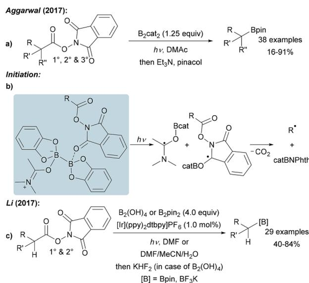
**Scheme 15** Decarboxylative borylation of alkyl carboxylic ester via the NHPI esters using  $B_2cat_2$  under blue LED irradiation (a) or with additional photo redox catalyst and  $B_2pin_2/B_2(OH)_4$  (c). Initiation (b).
