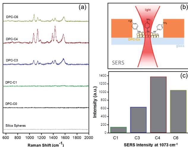
Fig. 7 (a) SERS of 4-aminothiophenol on plasmonic DPC-Cx, (b) SERS set-up, and (c) SERS intensities at 1073 cm<sup>-1</sup> using DPC-Cx.
