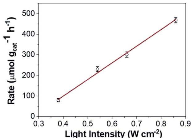
Fig. 10 Intensity-dependent photocatalytic rate of COL to CAL using DPC-C4.
