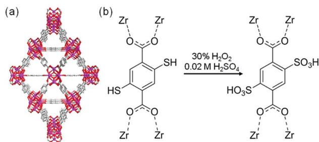
Fig. 8 (a) Crystal structure of UiO-66. (b) Scheme of the post-synthetic modification of UiO-66(SH)<sub>2</sub> to introduce sulfonic acid groups.
