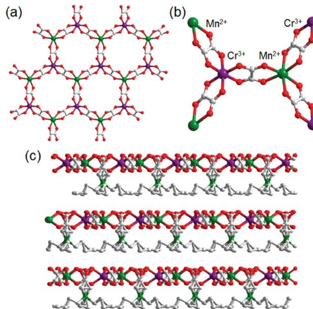
Fig. 5 The crystal structure of  $\{NR_3(CH_2COOH)\}-[MCr(ox)_3] \cdot nH_2O$ . (a) Representation of the coordination geometry around  $Mn^{II}$  and  $Cr^{III}$ , (b) the honeycomb layer structure, and (c) stacking view along the layers. Reproduced from ref. 49 with permission from American Chemical Society, Copyright 2012.
