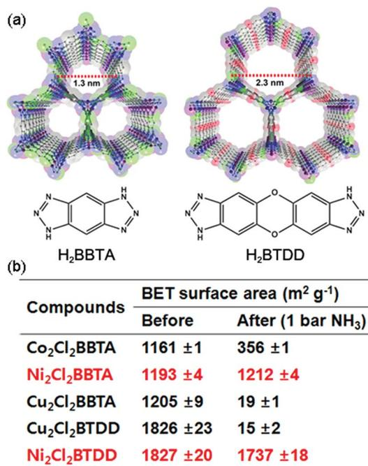
Fig. 13 (a) MOF structures based on H<sub>2</sub>BTDD (left) and H<sub>2</sub>BBTA (right) ligands. (b) Brunauer–Emmett–Teller (BET) surface area change after NH<sub>3</sub> exposure. Reproduced from ref. 66 with permission from American Chemical Society, Copyright 2018.
