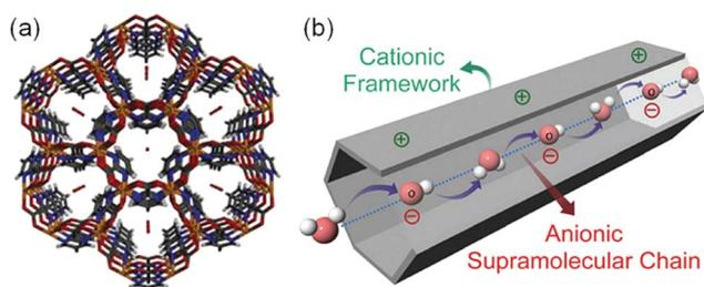
Fig. 11 (a) Crystal structure of [Ni<sub>2</sub>(m-pymca)<sub>3</sub>]OH·nH<sub>2</sub>O along the channel. (b) Schematic representation of a cationic MOF with an anionic supramolecular chain of hydroxide anions and water molecules inside the MOF pore for efficient hydroxide ion conduction. Reproduced from ref. 55 with permission from Royal Society of Chemistry, Copyright 2016.
