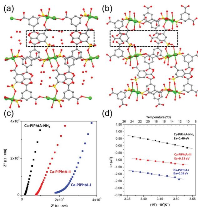
Fig. 16 *b*-axis view (*a*-axis horizontal) of the crystal structures of Ca-PiPhtA-I (a) and Ca-PiPhtA-II (b) showing the slightly different conformation of the 1-D channels along the *c* axis. (c) Plot of the complex impedance plane of Ca-PiPhtA compounds at 24 °C and 98% RH. (d) Arrhenius plots vs.  $T^{-1}$  from 10 to 24 °C. Reproduced from ref. 73 with permission from American Chemical Society, Copyright 2014.
