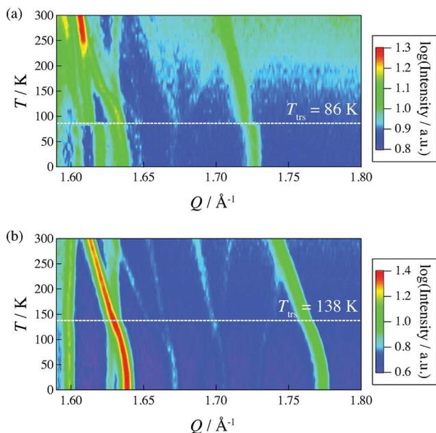
**Fig. 19** 2-D intensity maps obtained by neutron powder diffraction on IRIS for (a)  $(\text{NH}_4)_2(\text{adp})[\text{Zn}_2(\text{ox})_3] \cdot 3\text{H}_2\text{O}$  and (b)  $\text{K}_2(\text{adp})[\text{Zn}_2(\text{ox})_3] \cdot 3\text{H}_2\text{O}$ . The intensity is given on a logarithmic scale. The white dashed line represents each transition temperature. Reproduced with permission from ref. 77 with permission from Royal Society of Chemistry, Copyright 2014.
