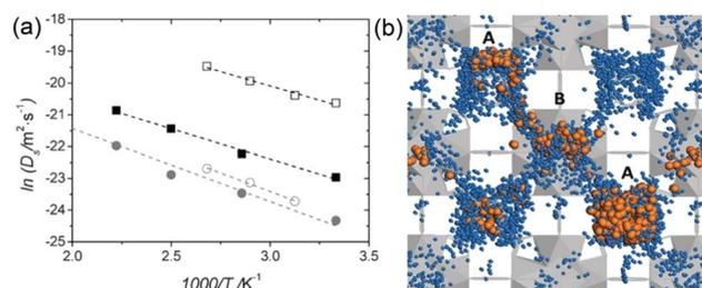
Fig. 23 (a) Arrhenius plot of  $D_s$  for protons (squares) and water molecules (circles) in the fully hydrated UiO-66(Zr)-(CO<sub>2</sub>H)<sub>2</sub>: QENS (open symbols) and aMS-EVB3-MD simulations (full symbols). (b) Illustration of simulation result for the water (blue)-mediated pathway with proton (orange) along the tetrahedral (A) and octahedral (B) cages of UiO-66(Zr)-(CO<sub>2</sub>H)<sub>2</sub> at 450 K. Reproduced from ref. 81 with permission from Wiley-VCH, Copyright 2016.
