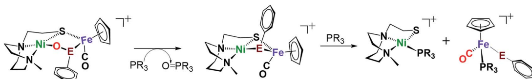
Fig. 7 Reaction of complex 2+O ( E = \text{Se} ) or 1+O ( E = \text{S} ) with O-abstrating agents, \text{PR}_3 ( R = \text{Me} or o\text{-tolyl} ).
