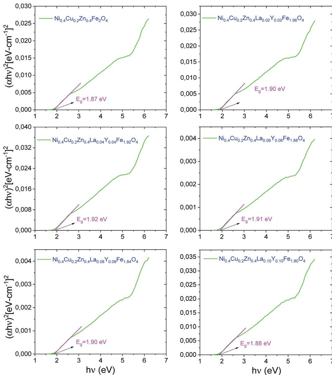
Fig. 6 Tauc plots and extrapolated direct  $E_g$  data of  $\text{Ni}_{0.4}\text{Cu}_{0.2}\text{Zn}_{0.4}\text{La}_x\text{Y}_x\text{Fe}_{2-x}\text{O}_4$  ( $x = 0.00 - 0.10$ ) NPs.
