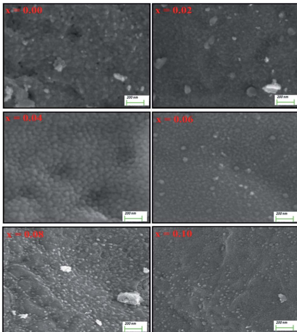
Fig. 2 SEM images of various  $\text{Ni}_{0.4}\text{Cu}_{0.2}\text{Zn}_{0.4}\text{La}_x\text{Y}_x\text{Fe}_{2-x}\text{O}_4$  ( $x = 0.00 - 0.10$ ) NSFs.
