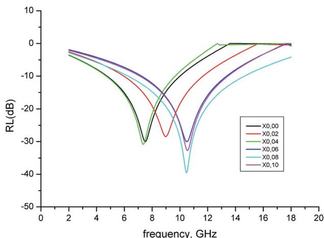
**Fig. 9** RL spectra of  $\text{Ni}_{0.4}\text{Cu}_{0.2}\text{Zn}_{0.4}\text{La}_x\text{Y}_x\text{Fe}_{2-x}\text{O}_4$  ( $x = 0.00 - 0.10$ ) NSFs.
