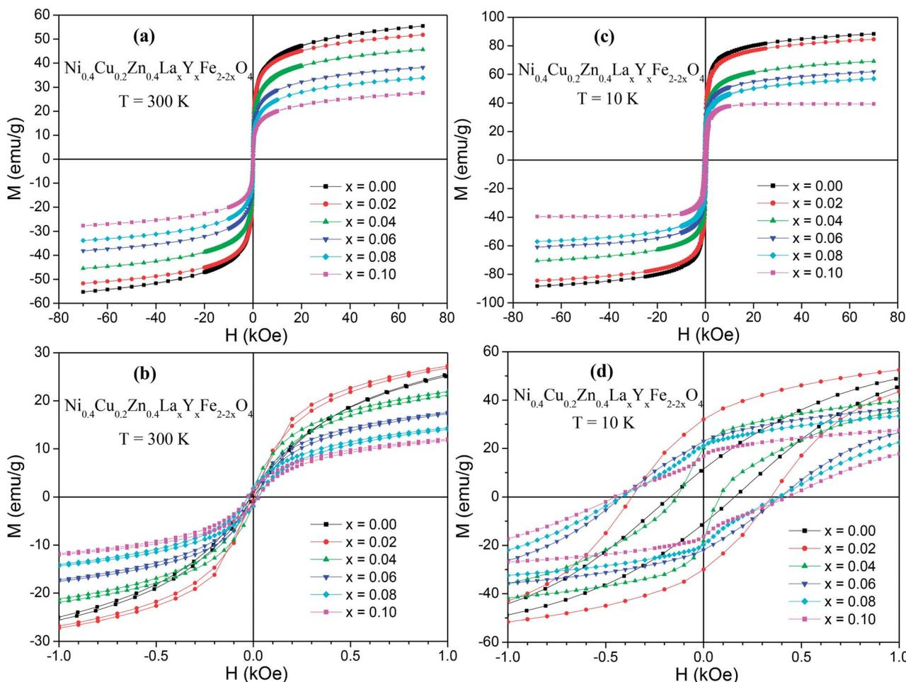
Fig. 8  $M$ - $H$  hysteresis loops of  $\text{Ni}_{0.4}\text{Cu}_{0.2}\text{Zn}_{0.4}\text{La}_x\text{Y}_x\text{Fe}_{2-2x}\text{O}_4$  ( $x = 0.00 - 0.10$ ) NSF $s$  performed at (a and b)  $T = 300$  and (c and d)  $T = 10$  K.
