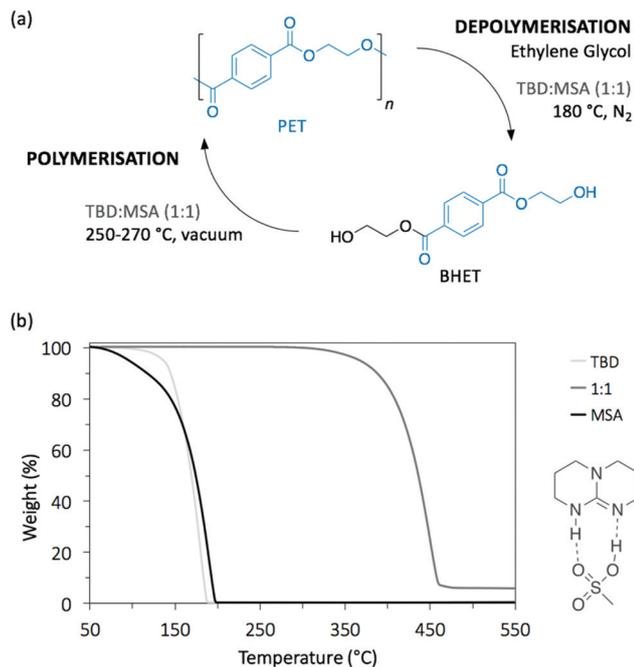
**Fig. 4** (a) The depolymerisation of PET and re-polymerisation of monomeric products (BHET) using TBD:MSA (1:1) catalyst and (b) the thermogravimetric analysis (TGA) comparison between TBD:MSA (1:1) and TBD and MSA alone.
