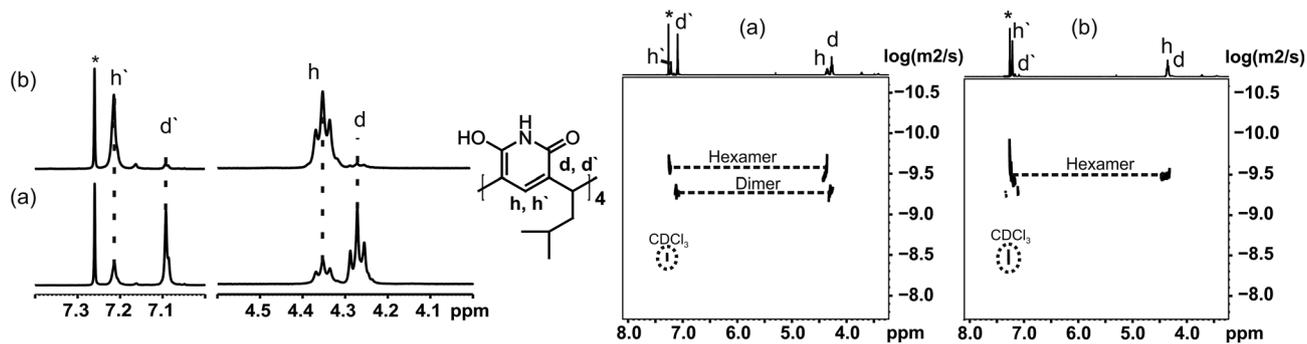
**Fig. 2** Left: <sup>1</sup>H NMR of **1** (20 mM in CDCl<sub>3</sub>) (a) measured within 2 hours after sample preparation and (b) same sample after 7 days from sample preparation. Right: DOSY NMR of the same sample (a) measured within 2 hours from sample preparation and (b) after 7 days from sample preparation. Signals d and d' correspond to the dimeric assembly and signals h and h' to the hexameric assembly.
