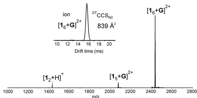
Fig. 1 (+)ESI-MS spectrum of **1** (60  $\mu$ M) and tris(bipyridine)ruthenium(II) (**G**) with 6 : 1 ratio measured from acetone/DCM mixture. Inset showing IMS arrival time distribution (ATD) for  $[1_6 + G]^{2+}$  ion.
