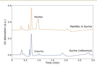
Fig. 4 UV chromatogram of the SFC separation of ManNac in Surine (top) (0.035 M, 0.5 μL injected volume) and pure Surine (bottom) on a 2-PIC column at 60 °C, 120 bar and a flow rate of 1.5 ml min $^{-1}$  for a mobile phase of 30% MeOH in CO $_2$ . A small impurity of a previous separation is present in the chromatogram of pure Surine. Under these conditions, ManNAc can be separated from synthetic urine.
