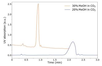
Fig. 3 UV chromatogram of the SFC separation of ManNac in water (0.78 M, 0.5  $\mu$ L injection volume) on a 2-PIC column (Waters) at 60 °C, 120 bar and a flow rate of 1.5 ml min<sup>-1</sup>. The top graph was separated with a mobile phase of 30% MeOH in CO<sub>2</sub>, and the bottom graph with 20% MeOH in CO<sub>2</sub>. The sharpest peak is obtained with 30% MeOH in CO<sub>2</sub>.
