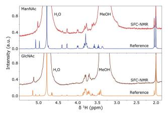
Fig. 7 SFC- $^1$ H NMR spectra of GlcNAc (bottom) and ManNAc (top) in D $_2$ O and MeOH, compared to their respective  $^1$ H NMR reference spectra (shown before in Fig. 6). The spectra were scaled to the integrals of the peak(s) around 2 ppm. A Lorentzian line broadening of 1.5 Hz was applied to the SFC-NMR spectra. The distinction between the two isomers is clearly visible in the SFC-NMR spectra.
