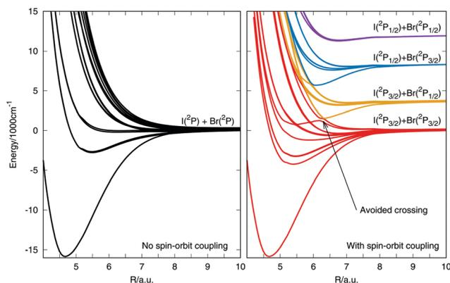
**Fig. 3** Potential energy curves of the IBr system. The left panel presents the 12 spin-free states dissociating to the ground states of I and Br. The right panel shows the 23 states when the spin–orbit coupling is considered.
