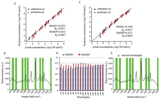
Fig. 8 (A) A linear regression plot of the calibration set and the prediction set for the ICPA built model; (B) the selected spectral intervals for the ICPA built model; (C) a linear regression plot of the calibration set and the prediction set for the ICPA-mRMR built model; (D) the changes of RMSEC and RMSEP with different numbers of wavelengths; (E) the distributions of selected wavelengths for the ICPA-mRMR built model.
