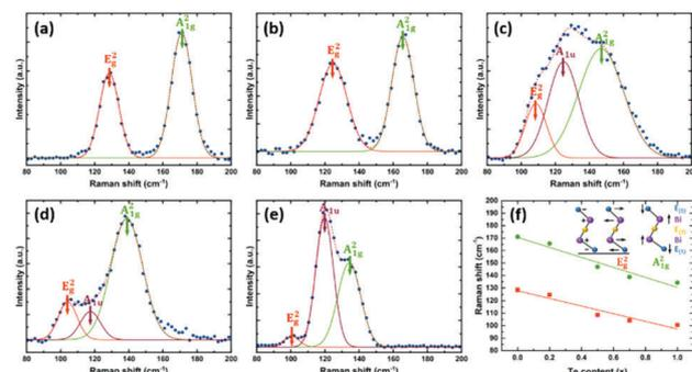
Fig. 5 (a–e) Raman spectra of as-deposited  $\text{Bi}_2(\text{Se}_{1-x}\text{Te}_x)_3$  films with  $x$  ranging from 0 to 1. (f) Phonon frequencies (orange:  $E_g^2$  mode; green:  $A_{1g}^2$  mode) as a function of Te composition. The inset provides the schematic diagrams for the two Raman-active modes.
