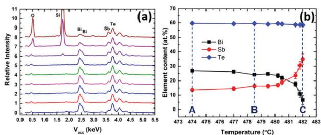
Fig. 6 (a) EDX spectra and (b) relationship between  $(\text{Bi}_{1-y}\text{Sb}_y)_2\text{Te}_3$  film composition and the increasing temperature of deposition (indicating the temperatures at positions A, B and C).
