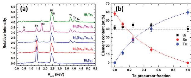
Fig. 2 (a) EDX spectra and (b) relationship between film composition and fraction of  $[\text{BiCl}_3(\text{Te}^n\text{Bu}_2)_3]$  used in the deposition of ternary  $\text{Bi}_2(\text{Se}_{1-x}\text{Te}_x)_3$  films.
