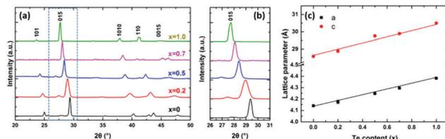
Fig. 4 (a) XRD patterns of as-deposited  $\text{Bi}_2(\text{Se}_{1-x}\text{Te}_x)_3$  films with  $x$  ranging from 0 to 1; (b) expanded XRD patterns showing the systematic shift of the 015 peak; (c) refined lattice parameters (see Table S1, ESI<sup>†</sup>) as a function of the Te content for different as-deposited  $\text{Bi}_2(\text{Se}_{1-x}\text{Te}_x)_3$  films.
