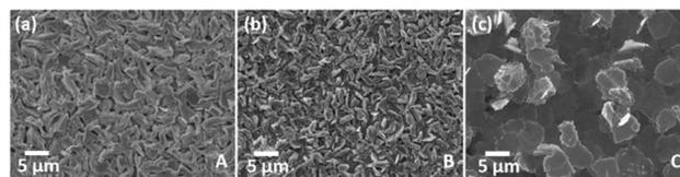
Fig. 7 SEM images of three regions (A–C) of the film deposited from a 1:1 ratio of  $[\text{SbCl}_3(\text{Te}^n\text{Bu}_2)_3]$  and  $[\text{BiCl}_3(\text{Te}^n\text{Bu}_2)_3]$  from Sb poor (a) to Sb rich (c).
