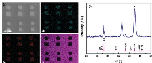
Fig. 1 (a) SEM image with EDX mapping and (b) grazing incidence XRD pattern from  $\text{Sb}_2\text{Te}_3$  selectively deposited from  $[\text{SbCl}_3(\text{Te}^n\text{Bu}_2)_3]$  into  $30\ \mu\text{m}$  TiN holes and an indexed bulk pattern of  $\text{Sb}_2\text{Te}_3$ .<sup>42</sup> The TiN substrate peaks are marked by \*.
