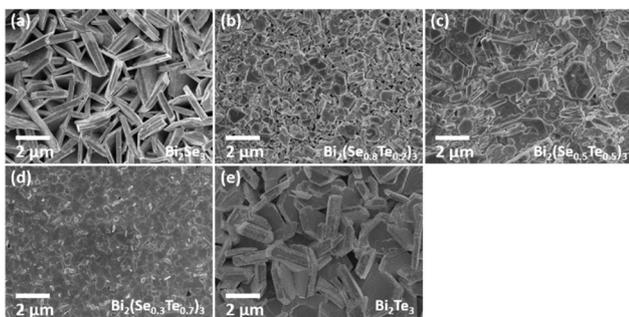
Fig. 3 SEM images showing the morphologies of the  $\text{Bi}_2\text{Se}_3$  (a),  $\text{Bi}_2\text{Te}_3$  (e) and ternary  $\text{Bi}_2(\text{Se}_{1-x}\text{Te}_x)_3$  (b–d) films deposited by LPCVD under similar conditions (550  $^\circ\text{C}/0.05$  mmHg) onto  $\text{SiO}_2$ -coated silicon substrates.
