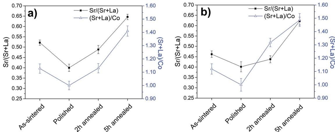
Fig. 4 Surface chemistry of LSC64 pellets characterized by (a) nano-probe AES and (b) XPS. The quantification shown from AES refers only to the particle free-regions of the LSC64 pellet surface.
